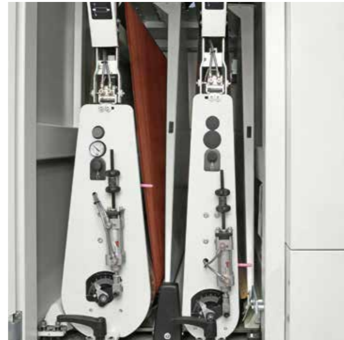
ON/OFF PNEUMATIC SELECTOR ON THE ROLLER UNIT It allows the roller exclusion from the sanding process while maintaining the working table position unchanged.
