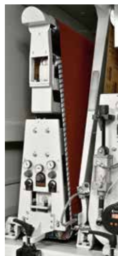
Superfinishing Unit with 2620 mm belt length.
