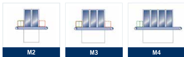
Available versions It is available in three versions, with two or three main operating units with 1350 mm working width. Excellent finishing results are obtained when machining raw and painted panels thanks to the wide range of units such as: Cross-Belt, Calibrating Roller, Sanding Roller, Superfinishing, Planetary and GSI-200 Brush.
