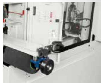
GSI-200 Brushing Unit for top machining versatility.
