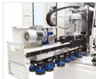
Planetary Unit: multi-directional sanding for maximum finishing.
