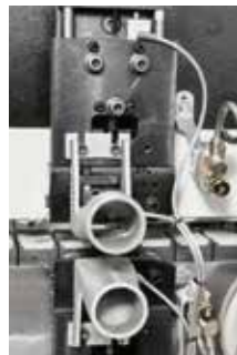
RC-N glue scraping unit It eliminates any glue excessing in the joint between edge and panel. Nesting processing.
