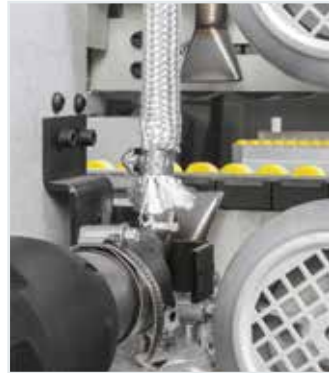
ID 3000 edge brightening unit It brightens the colour of plastic edges by heating them with hot air.
