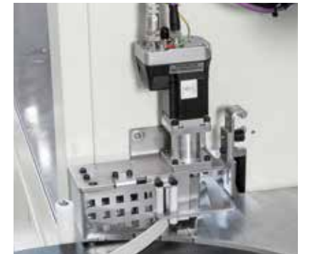
Kit for the automatic edge loading Fast, simple and safety edge changeover.
