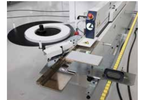
Infeed system for narrow pieces Simple, correct and safe panel insertion.
