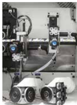
RAS-A edge scarping unit Simple and quick change of the machining radius with the replacement of the tool kit.
