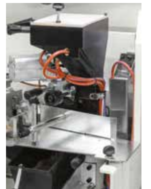
SGP-E glue pot Perfect joint line and use of EVA and PUR glue.
