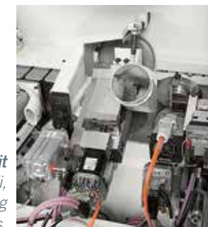
K-2 Radius end cutting unit Cut and radius in a single operation.
