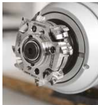
Round 2-A unit 2-motor unit and Multiedge device for processing 2 true radii.
