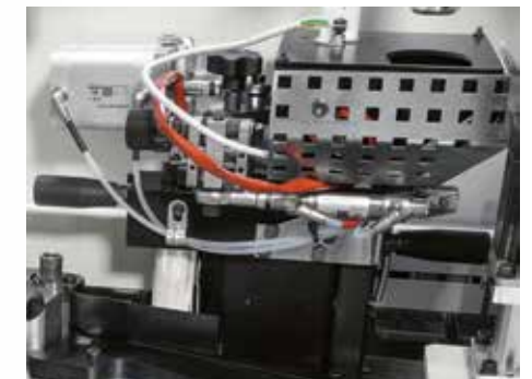
SGP glue pot Single device for EVA or PUR glue.
