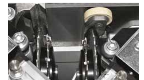
K-2 Radius end cutting unit Cut and radius in a single operation.
