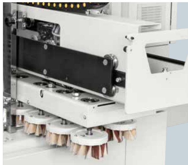
No machine down-time Extractable discs unit with sliding movement and rapid tools changeover system.
