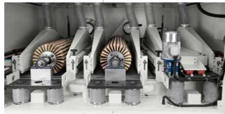
Available versions Two versions available, one for sanding with abrasive belts and the other for texturing with steel or tynex tools.
