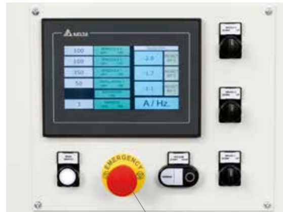
Maximum safety with the front and the two rear emergency stop push-buttons.
