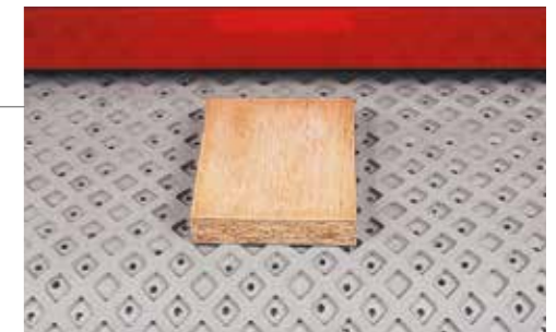
Natural rubber vacuum table with diamond-shaped belt, for the best piece traction.
