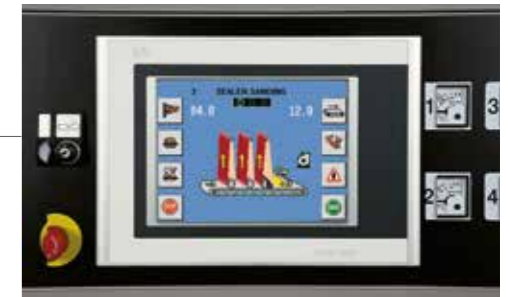
"Pro-sand" electronic programmer to control by the touch screen the automatic positioning of the units.
