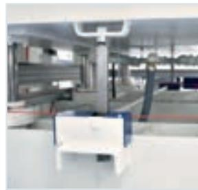
*Double rack and pinion system connected by a torsion bar to grant a flat movement of the press platen.*
