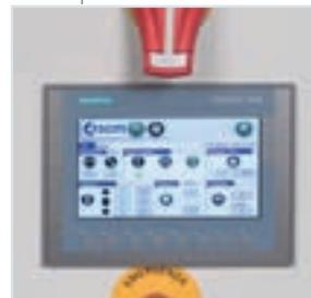
**Control panel with siemens colour touch screen**
