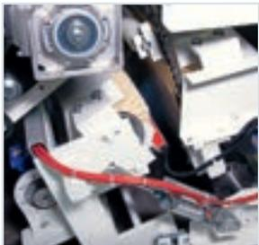
**Mylar belt ionizing unit** to repel dirt particles present in the environment. (optional)
