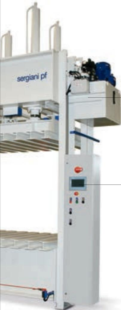
**Hydraulic unit** consists of a double pump and related electric motor dipped in hydraulic oil for a longer life and lower levels of noise. Automatic pressure loss recovery device ensures keeping the level set by the operator, in case of machined material failure.
